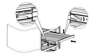
To remove a shelf, first remove the bottles and pull the shelf out to its limit. Depress the catch on the left hand sliding rail (see above), and at the same time lift the catch on the right hand sliding rail. The shelf may now be removed.
