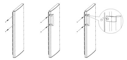
I: Remove two plug pins from 2: Fit the handle to the door the open side of the door. and fasten it with screws.
