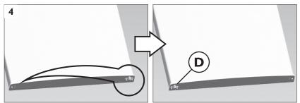
4. Remove the door limit block from the right side of the door end. Remove the blanking plate on the left side of the door end and screw the door limit block into that void. The finished item will look like (D).
