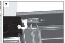
6. Set the door securely onto the bottom hinge in its new position. Support the door whilst you re-fit the top hinge (see step 7).
