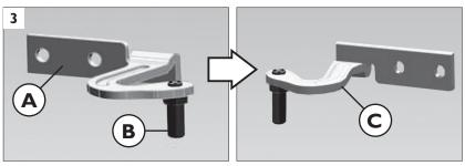
3. Take the top hinge (A) and flip it over. The door hinge mount (B) will then be pointing up. Disassemble the hinge mount with its nut and washer. Turn the hinge mount over so it is then pointing down and re-assemble into the top hinge. The finished item will look like (C).
