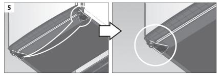
5. Tilt the appliance no more than 45° from vertical and use a hexagonal socket wrench to remove the screws that fix the bottom hinge to the unit. Move the bottom hinge to the left side of the unit and screw it into position.
