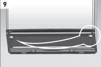
9. Move the levelling foot to the opposite side of the cabinet. Using a spirit level, adjust the foot until the unit is level and stable.
