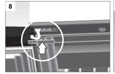
8. For a neat finish, fit the hinge cover over the void on the right side of the top panel.
